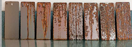
CorrosionX XD (far left) versus competitors after 120 hours in salt spray test
